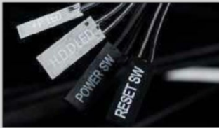
These four labelled cables connect your case's buttons and lights to the motherboard
