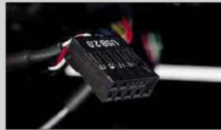
USB 2 connector - connects your board to your case's USB 2 ports
