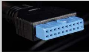
USB 3 connector - connects your motherboard to your case's USB 3 ports
